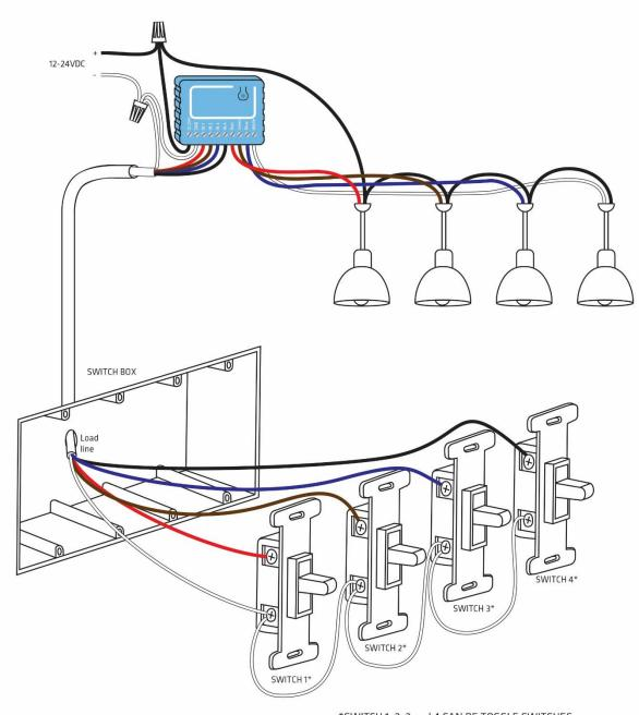
\*SWITCH 1, 2, 3 and 4 CAN BE TOGGLE SWITCHES, MOMENTARY SWITCHES OR TOGGLE WITH MEMORY SWITCHES. YOU MUST SET THE PARAMETERS TO THE RIGHT VALUE FOR DIFFERENT TYPES OF SWITCHES.
