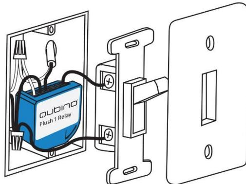
**INSTALLATION WITH ON/OFF SWITCH AND SCENE SWITCHES:**
