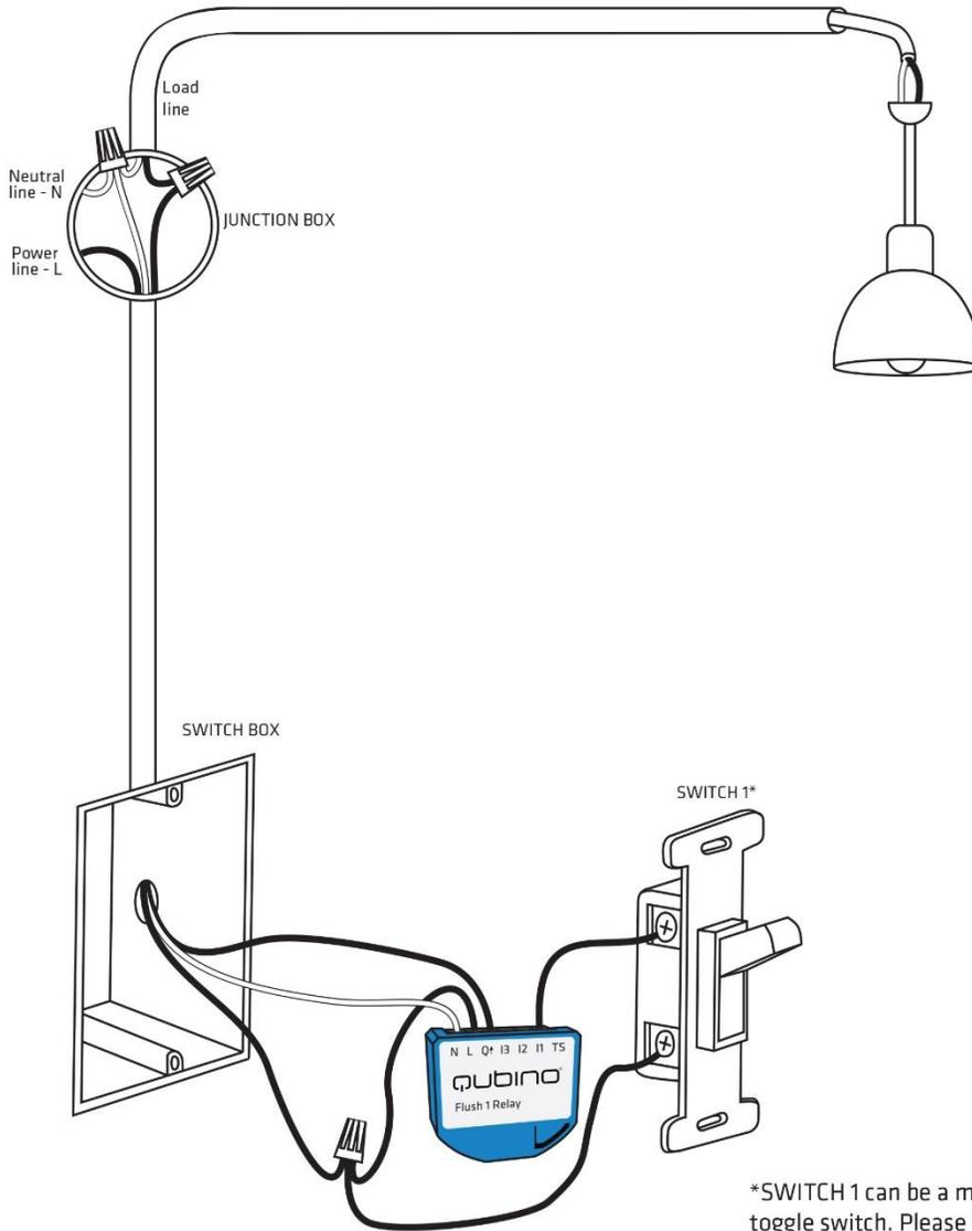
\*SWITCH 1 can be a momentary switch or a toggle switch. Please set parameter 1 to value 0 when connecting to a momentary switch. Set parameter 1 to value 1 when connecting to an on/off toggle switch (default setting). Please see the Configuration Parameters chapter for more information about advanced parameter settings.
