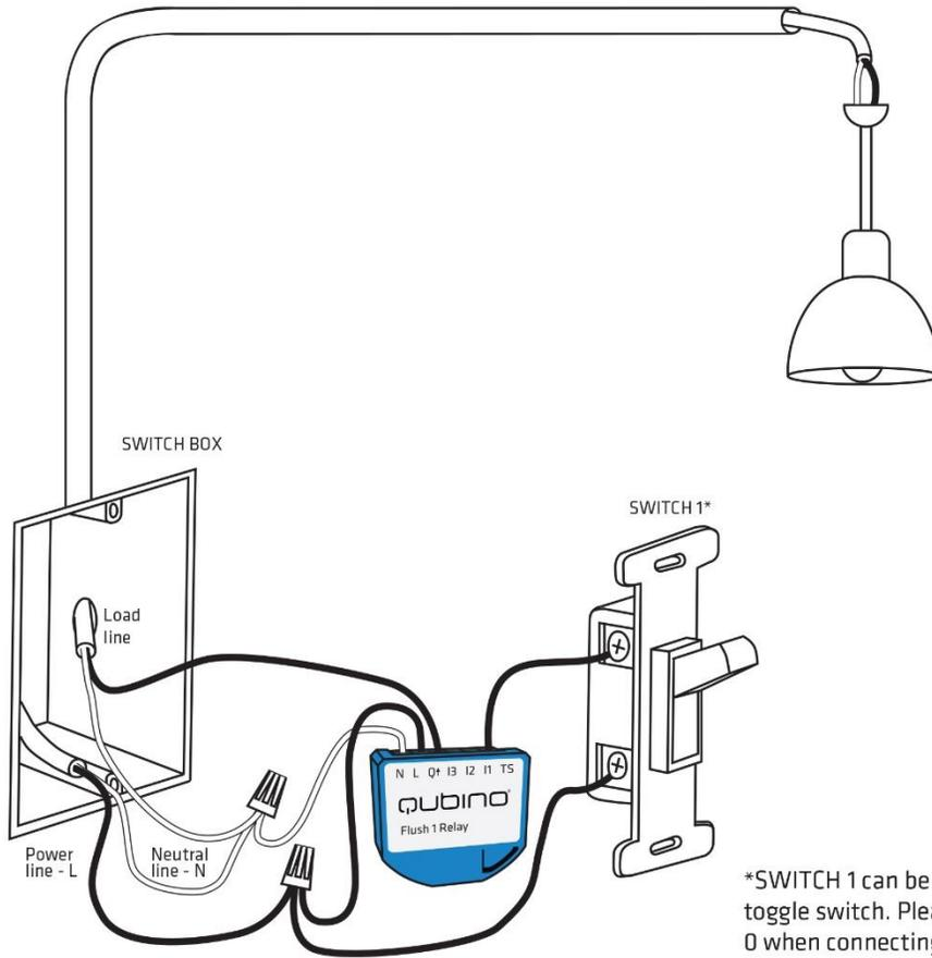
\*SWITCH 1 can be a momentary switch or a toggle switch. Please set parameter 1 to value 0 when connecting to a momentary switch. Set parameter 1 to value 1 when connecting to an on/off toggle switch (default setting). Please see the Configuration Parameters chapter for more information about advanced parameter settings
